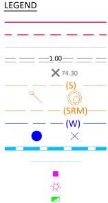
PROPERTY BOUNDARY EASEMENT EXISTING REVETMENT WALL (TOW RL. 1.0m) DESIGN CONTOURS (0.10m INTERVALS) FINISHED SURFACE LEVELS SEWER GRAVITY MAIN SEWER JUNCTION / MANHOLE SEWER RISING MAIN WATER MAIN (POTABLE) WATER HYDRANT / STOP VALVE STORMWATER DRAINAGE LOT STORMWATER OUTLET ELECTRICAL PILLAR STREET LIGHT NBN PIT
